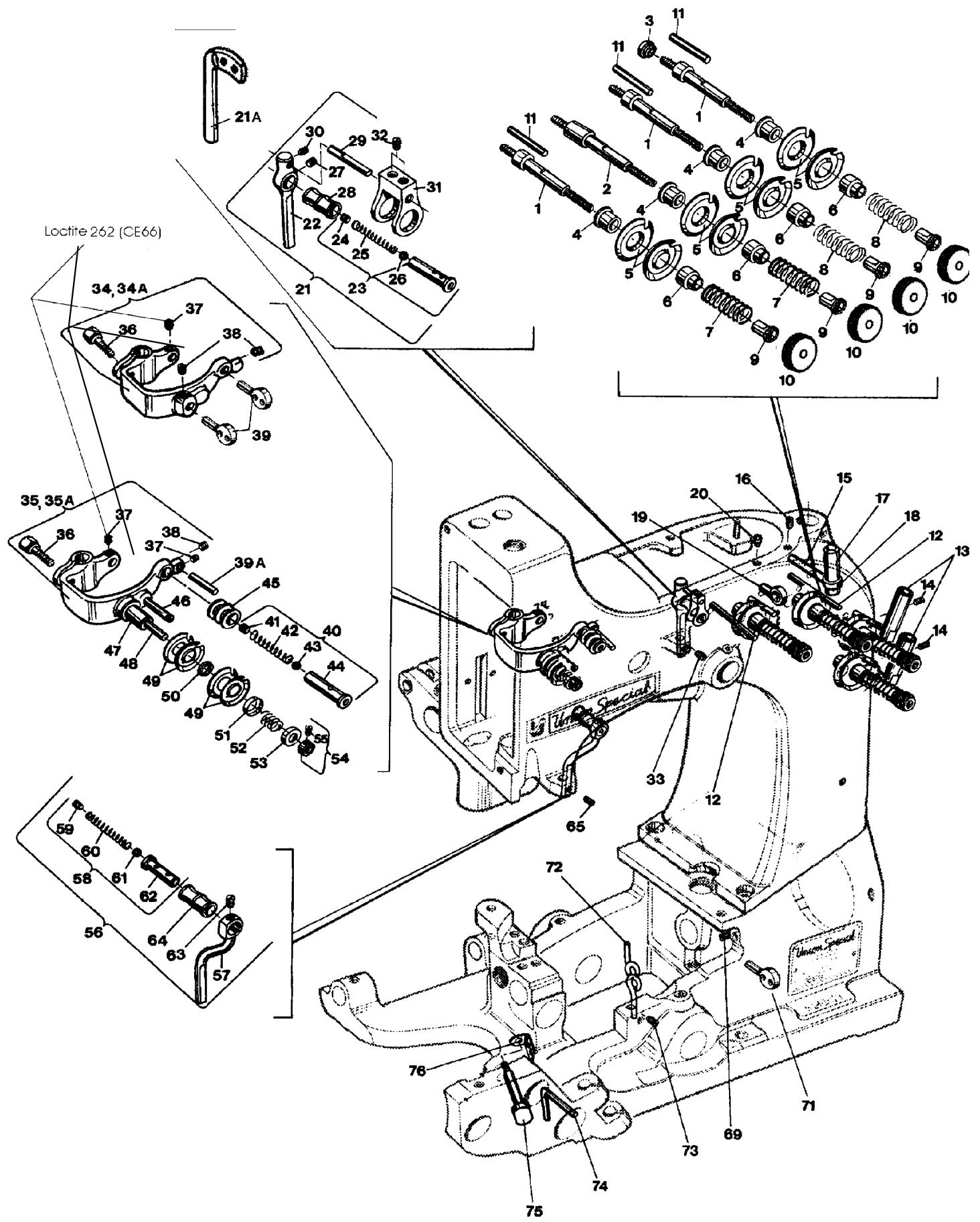
**THREAD TENSIONS AND THREAD GUIDE PARTS**
