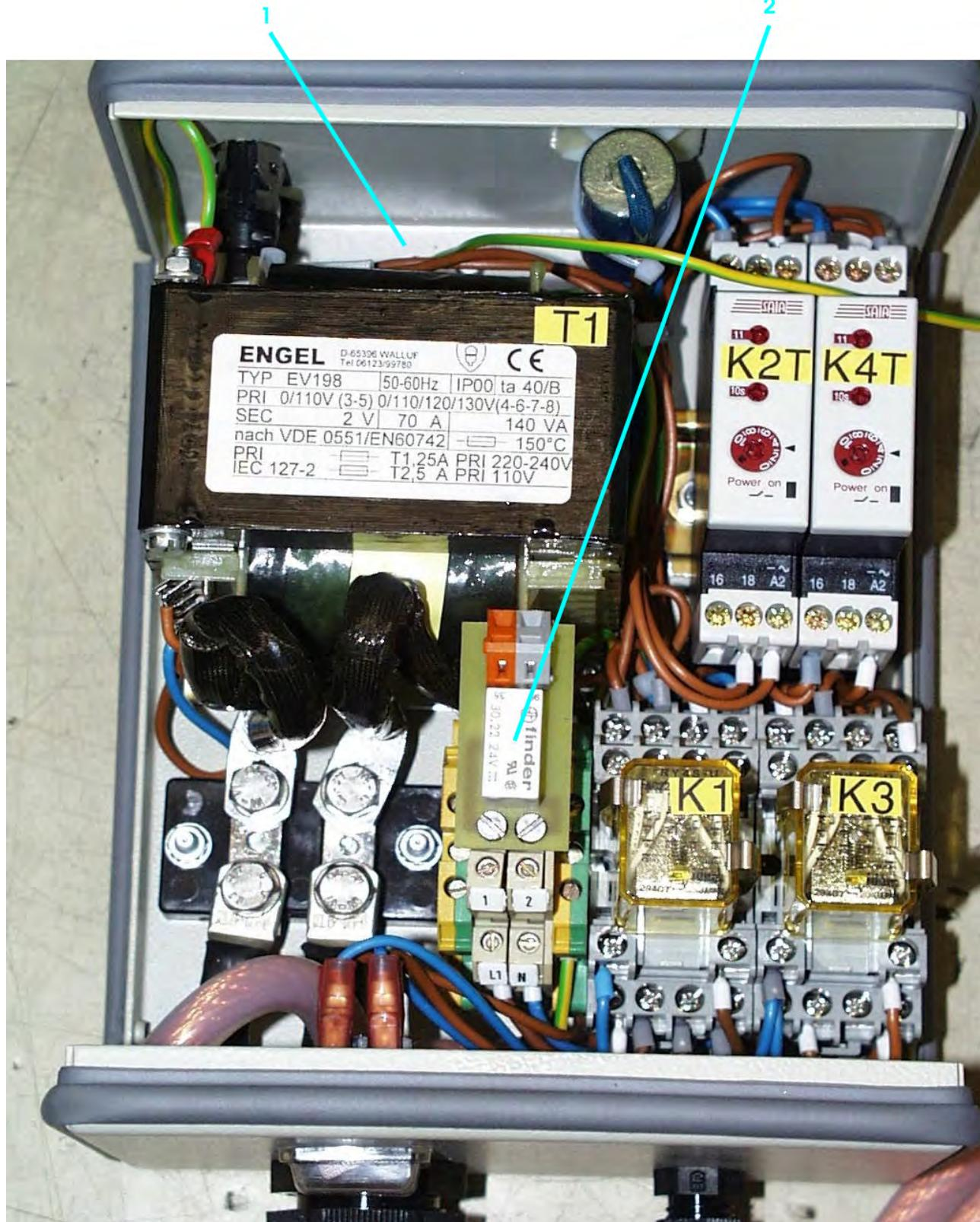
**CONTROL FOR ELECTRO-PNEUMATIC HOT THREAD CHAIN CUTTER 81300A1HLU, B1HLU**
