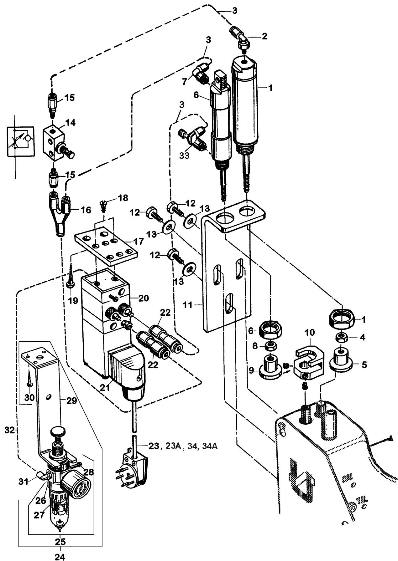
**ELECTRO-PNEUMATIC PARTS KIT FOR UPPER FEED PRESSURE AND LIFTER FOR 81300A1HLU, A2, B1HLU, B2
