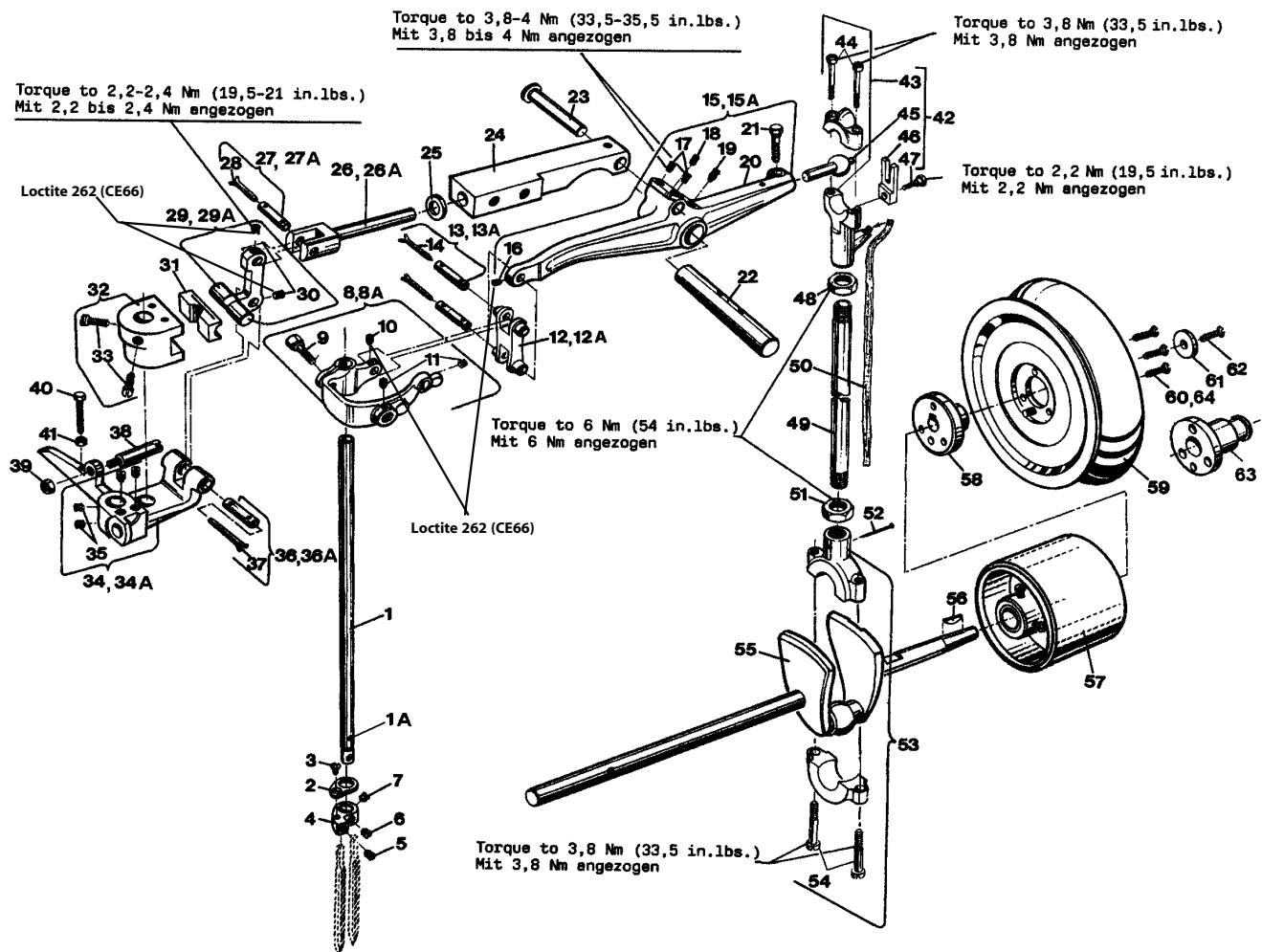
Shell of needle lever ball link should be positioned with an angle of  $7^{\circ} 48'$  in relation to the shell on the crankshaft.
