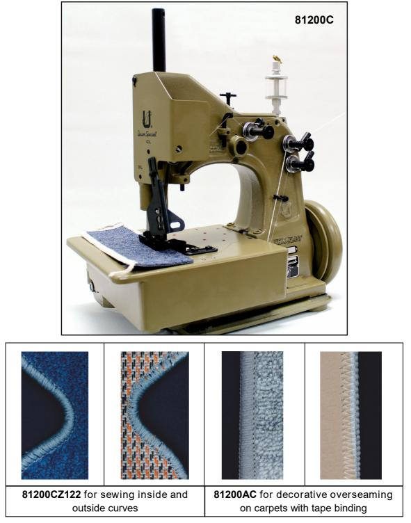
The 81200's Robust construction and Rugged reliability, combined with the ease of operation, will provide years of smooth long lasting service. Machines are available in two and three thread versions to serge a variety of styles and types of carpets, rugs and mats.
