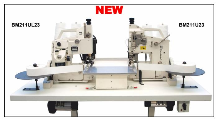
**BM211U23:** High performance single needle two thread double locked stitch sewing machine with vertical acting presser foot system and rust protected parts. For seaming and simultaneously tape binding left and right borders of building materials and geotextile layers. Tape respectively thread chain are automatically trimmed by an electro-pneumatically operated guillotine. Internal forced lubrication. Shell design casting. Low noise and vibration. Start-Stop controlled by photocell.
