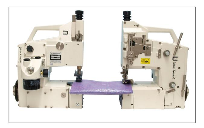
**BM211C:** High performance single needle two thread double locked stitch sewing machine with vertical acting presser foot system and rust protected parts. For seaming geotextile layers of fabric. With mechanically operated thread chain cutter. Internal forced lubrication. Shell design casting. Low noise and vibration.
