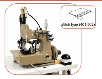
81300B, 81300B1HLU, 81300B2: Two needle safety stitch with top and bottom feed for matched seams on heavy bag fabrics
