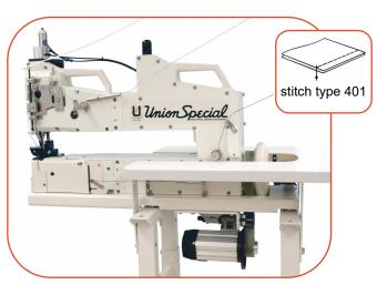
BML213C2: Longarm "POWERSTITCHER" Single needle double locked stitch with top and bottom feed for producing so called "Q"-inliner bags
