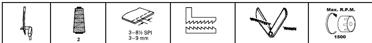
**Two thread chainstitch sewing machine with top and bottom feed with special sewing parts for fast, consistent joining of protection nets outdoors**
